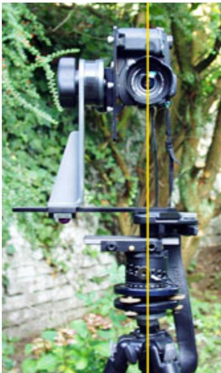
The centre of the lens and the rotating axis are on a same vertical line.
