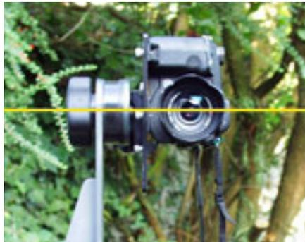
The centre of the lens and the tilting axis are on a same horizontal line.
